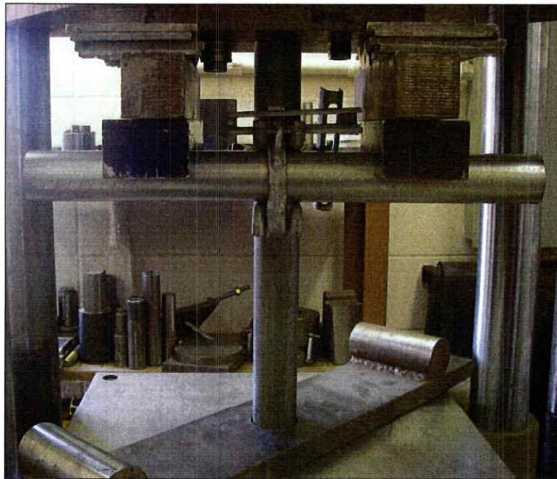
FIGURE 1 RIGHT ANGLE CLAMP TEST ARRANGEMENT
